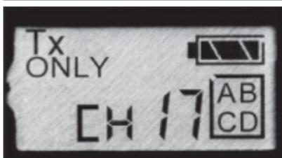
**Tx Only Mode** disables all receiving (**Rx**) functionality and allows you to use your Plus III as a transmitter only. Use this mode when sharing remote flashes with other photographers. This mode will prevent other photographers from triggering the Plus III on your camera.
