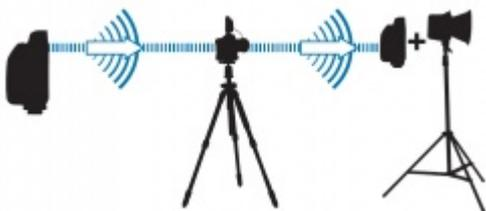
Auto Relay mode allows you to trigger remote flashes in sync with a remote camera and requires only three PocketWizard® radios. Using Auto Relay is the only situation where not all PocketWizard radios are set to the same Channel since the relaying radio triggers them one Channel higher than it received on. For more details about Relay Mode, please see the [Relay Mode](#) page.
