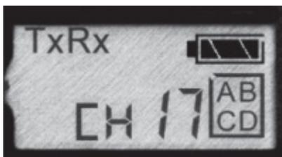
**TxRx Mode** allows the radio to be used as a transmitter attached to a camera or as a receiver connected to a remote flash or remote camera. As an Auto-Sensing Transceiver, the Plus III automatically switches between transmit and receive. This is the default mode.
