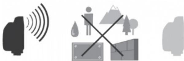
Your PocketWizard® radios use the environment as a medium for transmitting and receiving radio signals. The performance of your radios depends on their placement in the environment, nearby radio interference, and the radios' orientation and position relative to each other.
