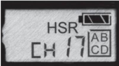
**HSR (High Speed Receive) Mode** shortens the contact time of the Flash/Camera Port, allowing for triggering of remote flashes at higher FPS (frames per second). This radio does not support HSS (High Speed Sync)
