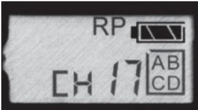
**RP (Repeater) Mode** allows you add one or more Plus III radio(s) between a pair of transmitting and receiving units to extend your range and increase the maximum triggering distance. This mode is recommended when triggering remote cameras. It can be used with flash with a reduction in maximum X-sync speed. This is not the same operation as Auto-Relay Mode
