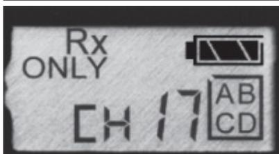
**Rx Only Mode** disables all transmit (Tx) functionality allowing you to use your Plus III radios as receivers for remote flashes or remote cameras. Use this mode when you do not want a remote Plus III to perform relay functions when mounted in the shoe of a remote camera, or to prevent a remote Plus III from triggering other radios when its TEST button is pressed.
