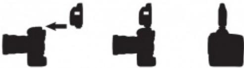
Connect a Plus III to your camera via the hot shoe. This will be your transmitting radio. Connect a Plus III to each of your remote flashes using the appropriate sync cable. These will be your receiving radios. If you are using a camera with no hot shoe, or the hot shoe cannot be used, connect the transmitting Plus III's Flash/Camera Port to the camera's sync terminal. Visit [our cablefinder](#) for correct camera cable.
