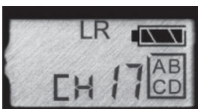
**LR (Long Range) Mode** dramatically increases the maximum range of a radio in a given shooting environment. Long Range Mode must be enabled on both transmitting and receiving radios. Use this mode when triggering remote cameras at greater distances. It can also be used with remote flash, but there may be a reduction in maximum X-sync speed.
